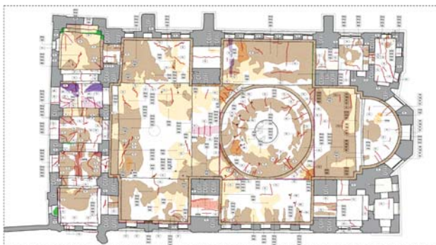
Hagia Irene Monument existing material decays, weak zones technical drawings
